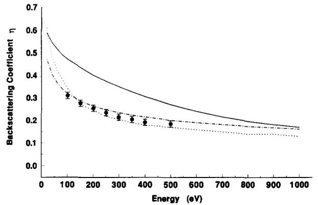
**Figure 2.** Experimental data (points with error bars) compared with simulations for the backscattering coefficient  $\eta$  as a function of incident electron energy. The optical data model (full curve) and the Liljequist corrected model (dotted curve) are two versions of the MC calculation. The predictions from the Verma empirical model are also shown (chain curve).
