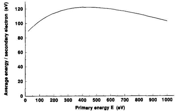
**Figure 5.** The average energy for generating a secondary electron as a function of primary energy. The parameters for the best fit were:  $U_0 = 85$  eV,  $\beta = -0.06$ ,  $\gamma = 80$  eV,  $E_0 = 280$  eV.
