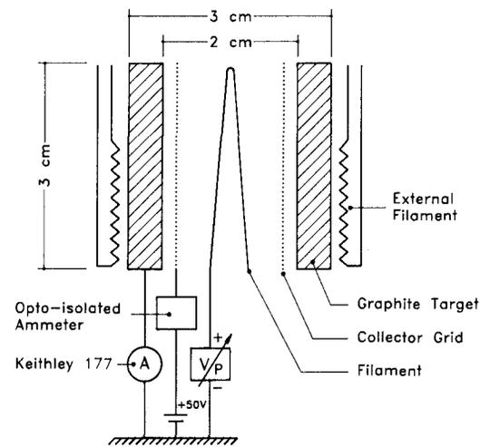
Figure 1. Schematic cross section of cylindrical triode used for measuring SEE yield  $\delta$ .
