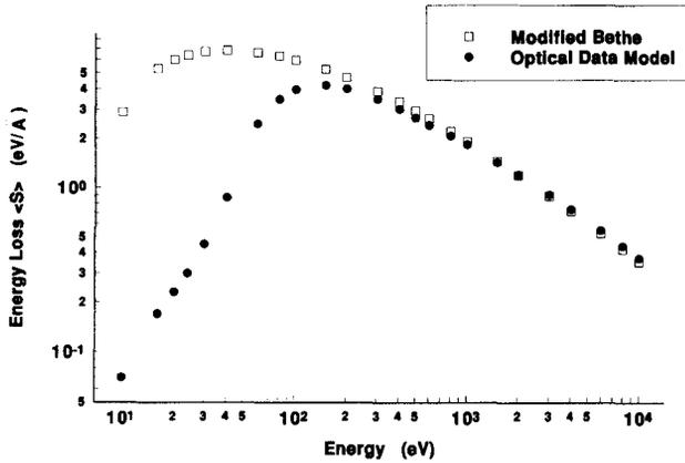
**Figure 4.** Electron energy loss as a function of electron energy in graphite according to the modified Bethe equation and an optical data model [14, 20].
