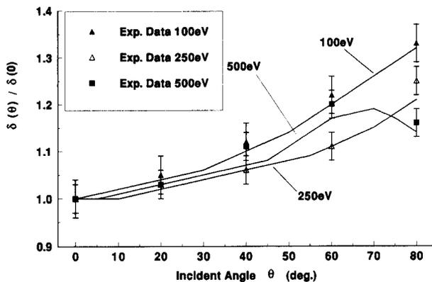
**Figure 7.** Experimental and theoretical SEE yield  $\delta$  as a function of the macroscopic angle of incidence of the primary electrons for three different primary electron energies. The data are from a solid carbon target with an optically rough surface [4].
