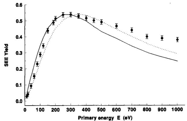
**Figure 3.** The comparison of the experimental SEE yield  $\delta$  (points with error bars), as a function of incident electron energy, with two simulation models. The optical data model (full curve) and the Liljequist corrected model (broken curve) are two versions of the MC calculation.
