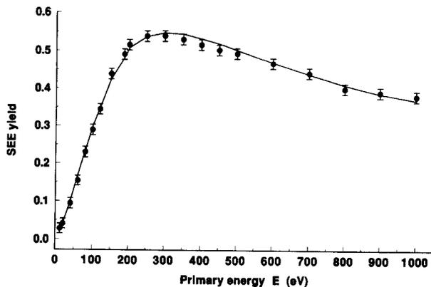
**Figure 6.** Comparison of the experimental data for the SEE yield  $\delta$  with a fitted simulation. The points with error bars represent the experimental data. The full curve shows the simulation result based on the fitted function of figure 5 for  $U$ .
